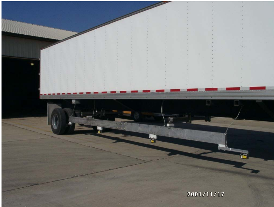
Figure 3. Aluminum beam with rear laser extended between the dual tires. (Note that the photo was taken prior to wrapping of the beam with thermal insulation.)
