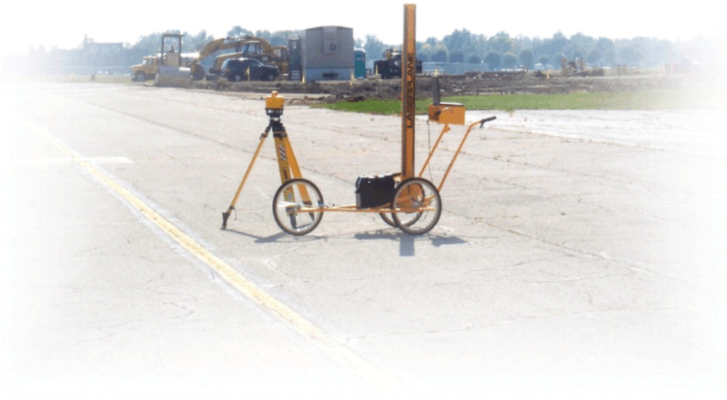
Figure 2. Picture of APR Consultants' Auto Rod and level.
