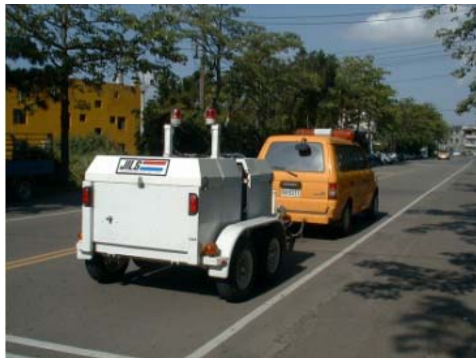
Figure 2 JILS-20 FWD Used in this Study
