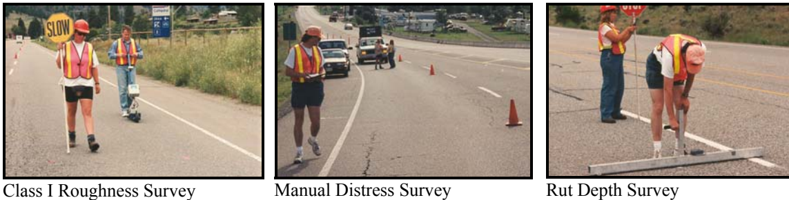
FIGURE 1 Advance manual surveys at initial QA site.
