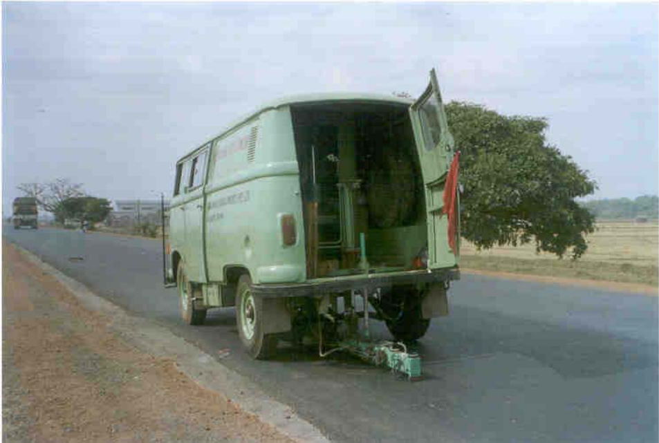
Figure 3 Field Evaluation of National Highway-6 using IITKGP FWD Model-II
