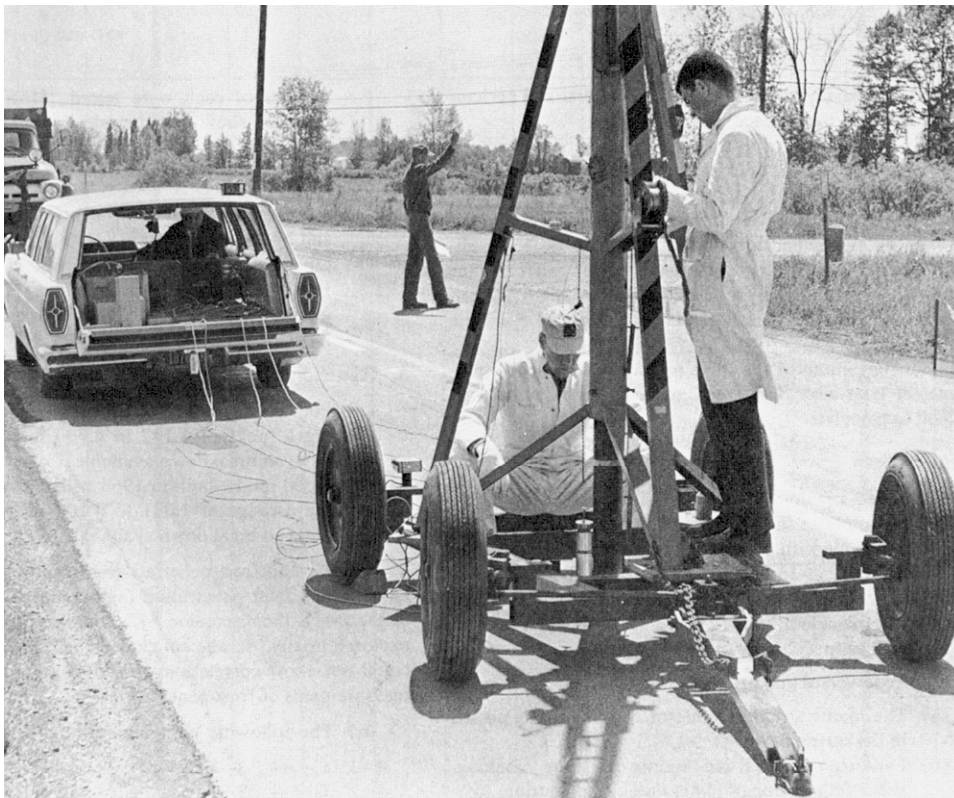
Figure 1. Road test with an early pulse loading system (Isada, 1966)
